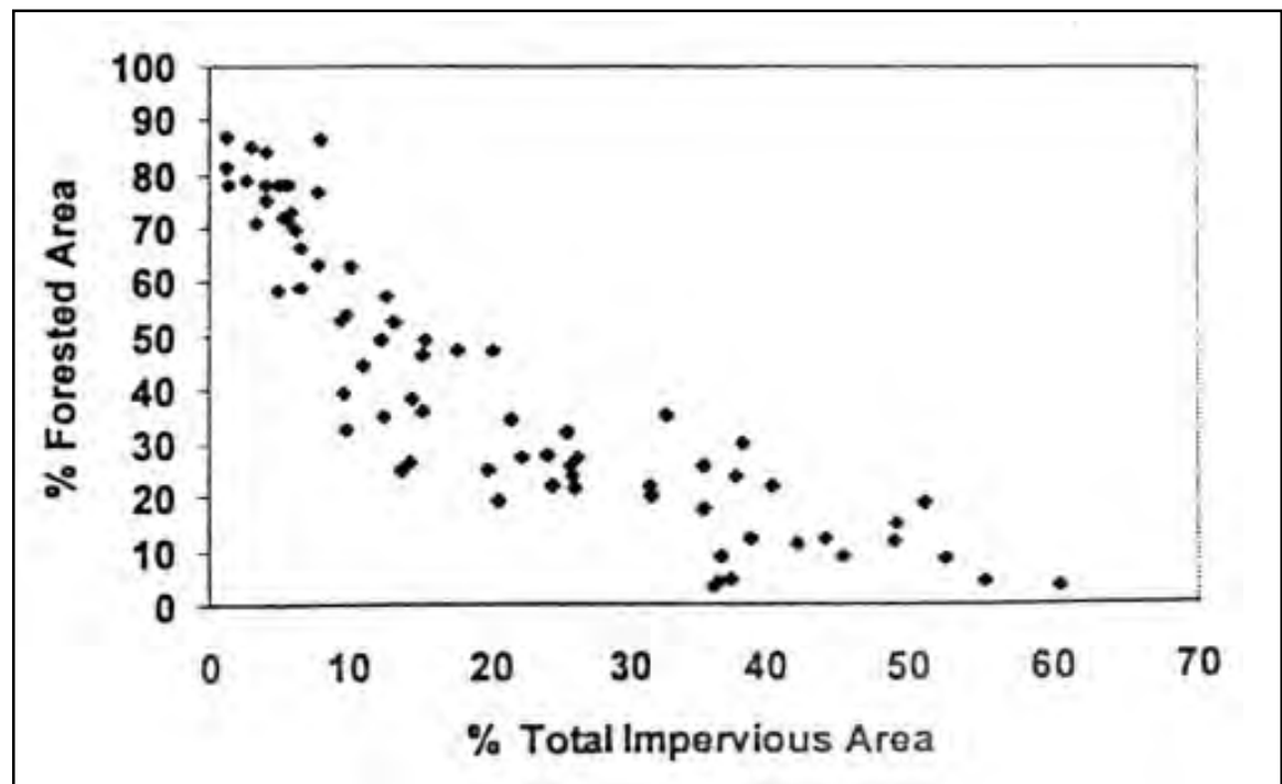
Figure 3: Relationship of IC and FC in Puget Sound Subwatersheds (Horner and May, 1999)
